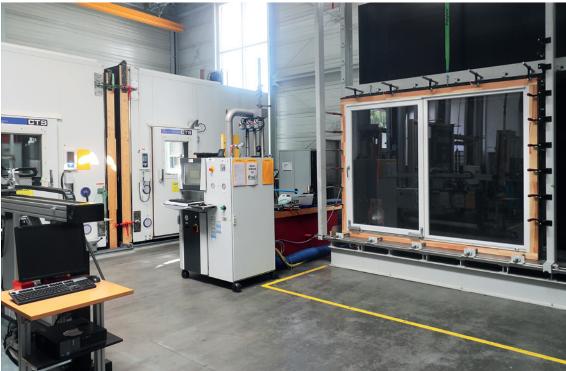
The Roto Test Centre at the headquarters in Leinfelden-Echterdingen is an accredited test laboratory where window manufacturers can have their systems tested. Here, the test for driving rain resistance is being carried out.
