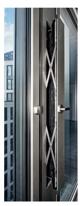
In addition to 4,200 Turn-Only windows with Roto AL Designo concealed hardware, 1675 parallel inward opening ventilation flaps were installed in the Marienturm in Frankfurt. These tightly sealed, easy-to-use ventilation flaps are equipped with parallel projecting scissor stays from the Roto PS Aintree range and special corner drives.
